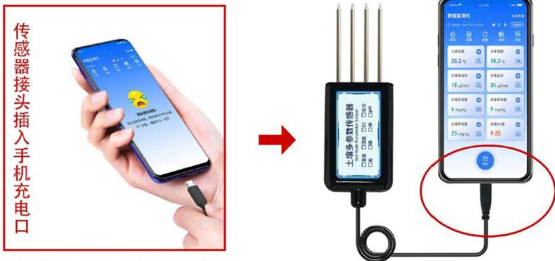
Insert the sensor connector into
