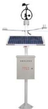
The sensor should be installed in an open area without any obstacles above the sensing surface
