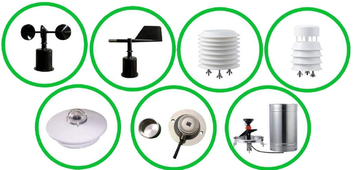
NBL-W-SS/The wind speed sensor adopts the traditional three-wind cup wind speed sensor structure, and the wind cup is made of carbon fiber material, which has high strength and good start-up; the built-in signal processing unit of the cup body can output the corresponding wind speed signal according to user needs.
